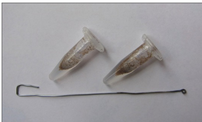
1.5 ml eppendorf caps with seeds and hypochlorite, and an inoculation loop made from a paper clip.
