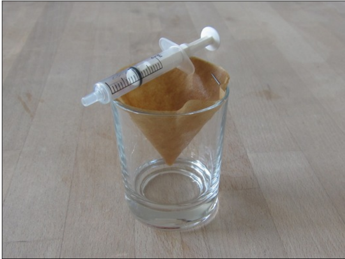
A home-made filter for removing sulfuric acid.
