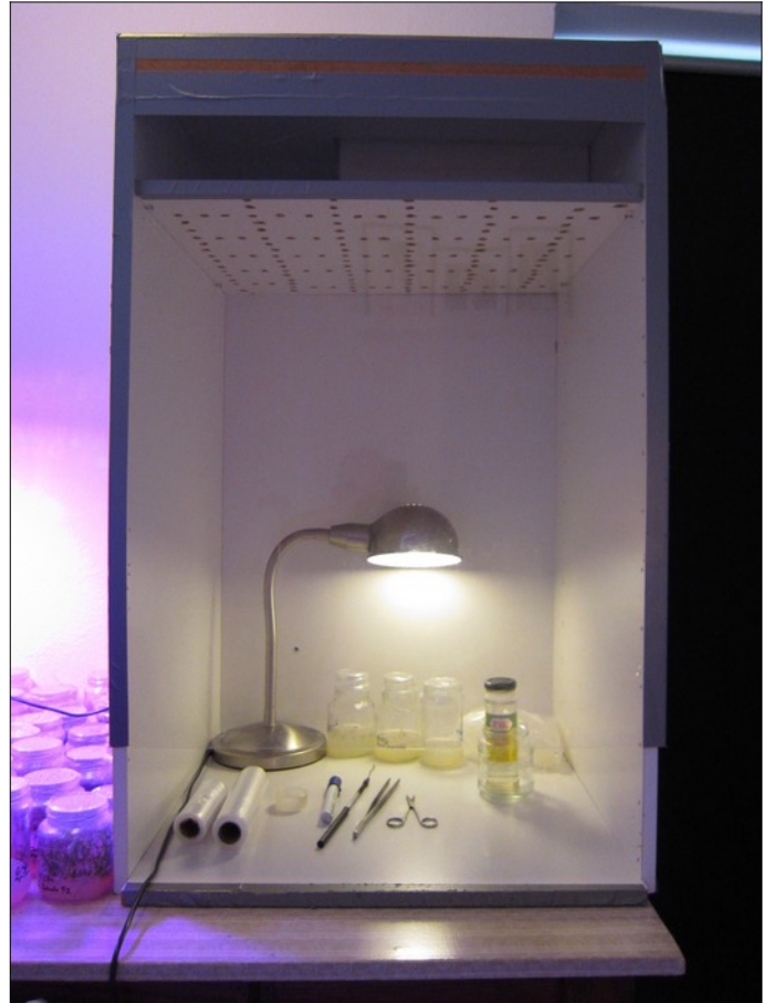
My home-made sterile cabinet, cheap, ugly, and very efficient. The dimensions are 60x60x80 cm. The opening is 15 cm.
